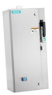
Non-reversing motor starter Size 0 Three phase full voltage Amb compensate bimetal OLrelay Contactor amp rating 18Amp 24VAC 50-60HZ coil Combination type 10Amp circuit breaker Encl NEMA type 4X 304 S-steel Water/dust tight noncorrosive Standard width enclosure
