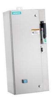
Non-reversing motor starter Size 0 Three phase full voltage Amb compensate bimetal OLrelay Contactor amp rating 18Amp 240V 50HZ / 277V 60HZ coil Combination type 10Amp circuit breaker Encl NEMA type 4X 304 S-steel Water/dust tight noncorrosive Standard width enclosure
