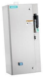
Non-reversing motor starter Size 0 Three phase full voltage Amb compensate bimetal OLrelay Contactor amp rating 18Amp 220-240/440-480VAC 60HZ coil Combination type 25Amp circuit breaker Encl NEMA type 4X 304 S-steel Water/dust tight noncorrosive Standard width enclosure
