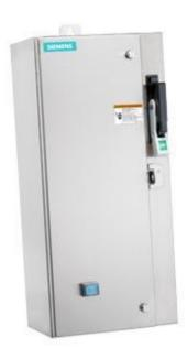
Non-reversing motor starter Size 0 Three phase full voltage Amb compensate bimetal OLrelay Contactor amp rating 18Amp 110V 50HZ / 120V 60HZ coil Combination type 25Amp circuit breaker Encl NEMA type 4X 304 S-steel Water/dust tight noncorrosive Standard width enclosure
