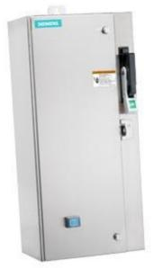
Non-reversing motor starter Size 0 Three phase full voltage Amb compensate bimetal OLrelay Contactor amp rating 18Amp 190-220/220-240V 50/60HZ coil Combination type 25Amp circuit breaker Encl NEMA type 4X 304 S-steel Water/dust tight noncorrosive Standard width enclosure
