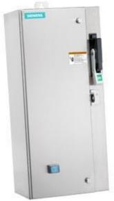
Non-reversing motor starter Size 0 Three phase full voltage Amb compensate bimetal OLrelay Contactor amp rating 18Amp 24VAC 50-60HZ coil Combination type 25Amp circuit breaker Encl NEMA type 4X 304 S-steel Water/dust tight noncorrosive Standard width enclosure
