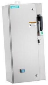
Non-reversing motor starter Size 0 Three phase full voltage Amb compensate bimetal OLrelay Contactor amp rating 18Amp 240V 50HZ / 277V 60HZ coil Combination type 25Amp circuit breaker Encl NEMA type 4X 304 S-steel Water/dust tight noncorrosive Standard width enclosure
