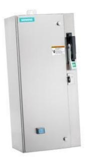
Non-reversing motor starter Size 0 Three phase full voltage Amb compensate bimetal OLrelay Contactor amp rating 18Amp 110-120/220-240VAC 60HZ coil Combination type 3Amp circuit breaker Encl NEMA type 4X 316 S-steel Water/dust tight noncorrosive Standard width enclosure
