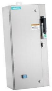
Non-reversing motor starter Size 0 Three phase full voltage Amb compensate bimetal OLrelay Contactor amp rating 18Amp 220-240/440-480VAC 60HZ coil Combination type 3Amp circuit breaker Encl NEMA type 4X 316 S-steel Water/dust tight noncorrosive Standard width enclosure
