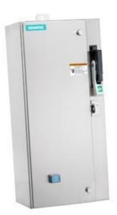
Non-reversing motor starter Size 0 Three phase full voltage Amb compensate bimetal OLrelay Contactor amp rating 18Amp 220-240/440-480VAC 60HZ coil Combination type 3Amp circuit breaker Encl NEMA type 4X 316 S-steel Water/dust tight noncorrosive Standard width enclosure
