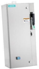
Non-reversing motor starter Size 0 Three phase full voltage Amb compensate bimetal OLrelay Contactor amp rating 18Amp 208VAC 60HZ coil Combination type 3Amp circuit breaker Encl NEMA type 4X 316 S-steel Water/dust tight noncorrosive Standard width enclosure
