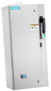
Non-reversing motor starter Size 0 Three phase full voltage Amb compensate bimetal OLrelay Contactor amp rating 18Amp 190-220/220-240V 50/60HZ coil Combination type 3Amp circuit breaker Encl NEMA type 4X 316 S-steel Water/dust tight noncorrosive Standard width enclosure
