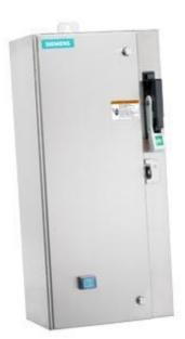
Non-reversing motor starter Size 0 Three phase full voltage Amb compensate bimetal OLrelay Contactor amp rating 18Amp 190-220/220-240V 50/60HZ coil Combination type 3Amp circuit breaker Encl NEMA type 4X 316 S-steel Water/dust tight noncorrosive Standard width enclosure
