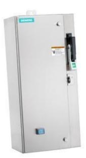
Non-reversing motor starter Size 0 Three phase full voltage Amb compensate bimetal OLrelay Contactor amp rating 18Amp 380-440/440-480V 50/60HZ coil Combination type 3Amp circuit breaker Encl NEMA type 4X 316 S-steel Water/dust tight noncorrosive Standard width enclosure
