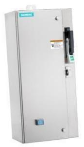
Non-reversing motor starter Size 0 Three phase full voltage Amb compensate bimetal OLrelay Contactor amp rating 18Amp 380-440/440-480V 50/60HZ coil Combination type 3Amp circuit breaker Encl NEMA type 4X 316 S-steel Water/dust tight noncorrosive Standard width enclosure
