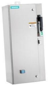
Non-reversing motor starter Size 0 Three phase full voltage Amb compensate bimetal OLrelay Contactor amp rating 18Amp 24VAC 50-60HZ coil Combination type 3Amp circuit breaker Encl NEMA type 4X 316 S-steel Water/dust tight noncorrosive Standard width enclosure
