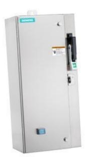
Non-reversing motor starter Size 0 Three phase full voltage Amb compensate bimetal OLrelay Contactor amp rating 18Amp 24VAC 50-60HZ coil Combination type 3Amp circuit breaker Encl NEMA type 4X 316 S-steel Water/dust tight noncorrosive Standard width enclosure
