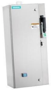
Non-reversing motor starter Size 0 Three phase full voltage Amb compensate bimetal OLrelay Contactor amp rating 18Amp 240V 50HZ / 277V 60HZ coil Combination type 3Amp circuit breaker Encl NEMA type 4X 316 S-steel Water/dust tight noncorrosive Standard width enclosure
