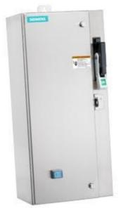
Non-reversing motor starter Size 0 Three phase full voltage Amb compensate bimetal OLrelay Contactor amp rating 18Amp 208VAC 60HZ coil Combination type 10Amp circuit breaker Encl NEMA type 4X 316 S-steel Water/dust tight noncorrosive Standard width enclosure
