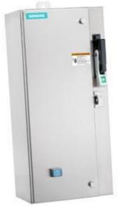
Non-reversing motor starter Size 0 Three phase full voltage Amb compensate bimetal OLrelay Contactor amp rating 18Amp 110V 50HZ / 120V 60HZ coil Combination type 10Amp circuit breaker Encl NEMA type 4X 316 S-steel Water/dust tight noncorrosive Standard width enclosure
