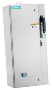
Non-reversing motor starter Size 0 Three phase full voltage Amb compensate bimetal OLrelay Contactor amp rating 18Amp 190-220/220-240V 50/60HZ coil Combination type 10Amp circuit breaker Encl NEMA type 4X 316 S-steel Water/dust tight noncorrosive Standard width enclosure
