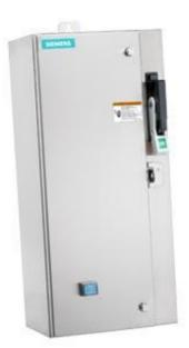
Non-reversing motor starter Size 0 Three phase full voltage Amb compensate bimetal OLrelay Contactor amp rating 18Amp 380-440/440-480V 50/60HZ coil Combination type 10Amp circuit breaker Encl NEMA type 4X 316 S-steel Water/dust tight noncorrosive Standard width enclosure
