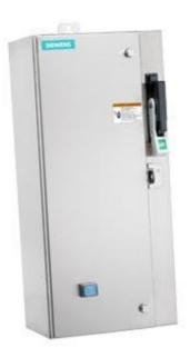
Non-reversing motor starter Size 0 Three phase full voltage Amb compensate bimetal OLrelay Contactor amp rating 18Amp 110-120/220-240VAC 60HZ coil Combination type 25Amp circuit breaker Encl NEMA type 4X 316 S-steel Water/dust tight noncorrosive Standard width enclosure
