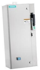
Non-reversing motor starter Size 0 Three phase full voltage Amb compensate bimetal OLrelay Contactor amp rating 18Amp 110-120/220-240VAC 60HZ coil Combination type 25Amp circuit breaker Encl NEMA type 4X 316 S-steel Water/dust tight noncorrosive Standard width enclosure
