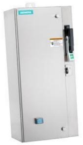
Non-reversing motor starter Size 0 Three phase full voltage Amb compensate bimetal OLrelay Contactor amp rating 18Amp 110V 50HZ / 120V 60HZ coil Combination type 25Amp circuit breaker Encl NEMA type 4X 316 S-steel Water/dust tight noncorrosive Standard width enclosure
