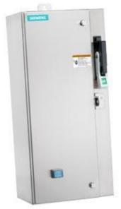
Non-reversing motor starter Size 0 Three phase full voltage Amb compensate bimetal OLrelay Contactor amp rating 18Amp 190-220/220-240V 50/60HZ coil Combination type 25Amp circuit breaker Encl NEMA type 4X 316 S-steel Water/dust tight noncorrosive Standard width enclosure
