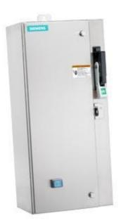
Non-reversing motor starter Size 0 Three phase full voltage Amb compensate bimetal OLrelay Contactor amp rating 18Amp 24VAC 50-60HZ coil Combination type 25Amp circuit breaker Encl NEMA type 4X 316 S-steel Water/dust tight noncorrosive Standard width enclosure
