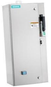
Non-reversing motor starter Size 0 Three phase full voltage Amb compensate bimetal OLrelay Contactor amp rating 18Amp 240V 50HZ / 277V 60HZ coil Combination type 25Amp circuit breaker Encl NEMA type 4X 316 S-steel Water/dust tight noncorrosive Standard width enclosure
