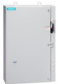
Non-reversing motor starter Size 0 Three phase full voltage Solidstate overload relay OLRelay amp range 0.75-3.4A 220-240/440-480VAC 60HZ coil Combination type 3Amp circuit breaker Encl NEMA type 4X 316 S-steel Water/dust tight noncorrosive Extra-wide enclosure
