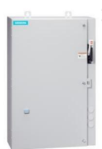
Non-reversing motor starter Size 0 Three phase full voltage Solidstate overload relay OLRelay amp range 0.75-3.4A 110V 50HZ / 120V 60HZ coil Combination type 3Amp circuit breaker Encl NEMA type 4X 316 S-steel Water/dust tight noncorrosive Extra-wide enclosure
