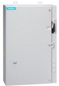
Non-reversing motor starter Size 0 Three phase full voltage Solidstate overload relay OLRelay amp range 0.75-3.4A 190-220/220-240V 50/60HZ coil Combination type 3Amp circuit breaker Encl NEMA type 4X 316 S-steel Water/dust tight noncorrosive Extra-wide enclosure
