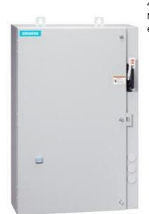
Non-reversing motor starter Size 0 Three phase full voltage Solidstate overload relay OLRelay amp range 0.75-3.4A 380-440/440-480V 50/60HZ coil Combination type 3Amp circuit breaker Encl NEMA type 4X 316 S-steel Water/dust tight noncorrosive Extra-wide enclosure
