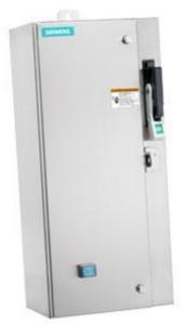
Non-reversing motor starter Size 0 Three phase full voltage Solidstate overload relay OLRelay amp range 0.75-3.4A 110V 50HZ / 120V 60HZ coil Combination type 3Amp circuit breaker Encl NEMA type 4X 304 S-steel Water/dust tight noncorrosive Standard width enclosure
