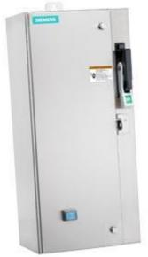
Non-reversing motor starter Size 0 Three phase full voltage Solidstate overload relay OLRelay amp range 0.75-3.4A 220-240/440-480VAC 60HZ coil Combination type 3Amp circuit breaker Encl NEMA type 4X 316 S-steel Water/dust tight noncorrosive Standard width enclosure
