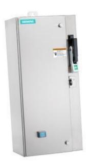
Non-reversing motor starter Size 0 Three phase full voltage Solidstate overload relay OLRelay amp range 0.75-3.4A 110V 50HZ / 120V 60HZ coil Combination type 3Amp circuit breaker Encl NEMA type 4X 316 S-steel Water/dust tight noncorrosive Standard width enclosure
