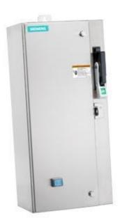
Non-reversing motor starter Size 0 Three phase full voltage Solidstate overload relay OLRelay amp range 0.75-3.4A 240V 50HZ / 277V 60HZ coil Combination type 3Amp circuit breaker Encl NEMA type 4X 316 S-steel Water/dust tight noncorrosive Standard width enclosure
