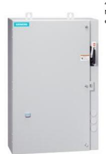
Non-reversing motor starter Size 0 Three phase full voltage Solidstate overload relay OLRelay amp range 3-12A 220-240/440-480VAC 60HZ coil Combination type 10Amp circuit breaker Encl NEMA type 4X 316 S-steel Water/dust tight noncorrosive Extra-wide enclosure
