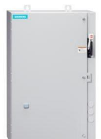
Non-reversing motor starter Size 0 Three phase full voltage Solidstate overload relay OLRelay amp range 3-12A 240V 50HZ / 277V 60HZ coil Combination type 10Amp circuit breaker Encl NEMA type 4X 316 S-steel Water/dust tight noncorrosive Extra-wide enclosure
