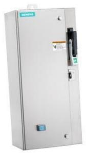
Non-reversing motor starter Size 0 Three phase full voltage Solidstate overload relay OLRelay amp range 3-12A 110V 50HZ / 120V 60HZ coil Combination type 10Amp circuit breaker Encl NEMA type 4X 304 S-steel Water/dust tight noncorrosive Standard width enclosure
