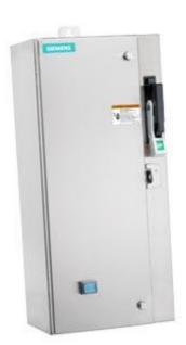
Non-reversing motor starter Size 0 Three phase full voltage Solidstate overload relay OLRelay amp range 3-12A 110-120/220-240VAC 60HZ coil Combination type 10Amp circuit breaker Encl NEMA type 4X 316 S-steel Water/dust tight noncorrosive Standard width enclosure
