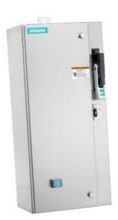
Non-reversing motor starter Size 0 Three phase full voltage Solidstate overload relay OLRelay amp range 3-12A 220-240/440-480VAC 60HZ coil Combination type 10Amp circuit breaker Encl NEMA type 4X 316 S-steel Water/dust tight noncorrosive Standard width enclosure
