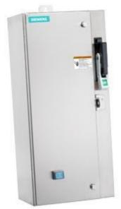
Non-reversing motor starter Size 0 Three phase full voltage Solidstate overload relay OLRelay amp range 3-12A 208VAC 60HZ coil Combination type 10Amp circuit breaker Encl NEMA type 4X 316 Ssteel Water/dust tight noncorrosive Standard width enclosure
