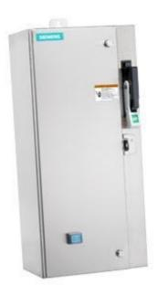
Non-reversing motor starter Size 0 Three phase full voltage Solidstate overload relay OLRelay amp range 3-12A 110V 50HZ / 120V 60HZ coil Combination type 10Amp circuit breaker Encl NEMA type 4X 316 S-steel Water/dust tight noncorrosive Standard width enclosure
