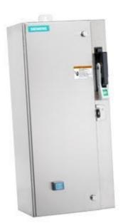
Non-reversing motor starter Size 0 Three phase full voltage Solidstate overload relay OLRelay amp range 3-12A 190-220/220-240V 50/60HZ coil Combination type 10Amp circuit breaker Encl NEMA type 4X 316 S-steel Water/dust tight noncorrosive Standard width enclosure
