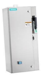
Non-reversing motor starter Size 0 Three phase full voltage Solidstate overload relay OLRelay amp range 3-12A 380-440/440-480V 50/60HZ coil Combination type 10Amp circuit breaker Encl NEMA type 4X 316 S-steel Water/dust tight noncorrosive Standard width enclosure
