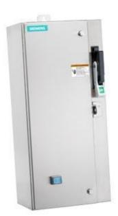
Non-reversing motor starter Size 0 Three phase full voltage Solidstate overload relay OLRelay amp range 3-12A 240V 50HZ / 277V 60HZ coil Combination type 10Amp circuit breaker Encl NEMA type 4X 316 S-steel Water/dust tight noncorrosive Standard width enclosure
