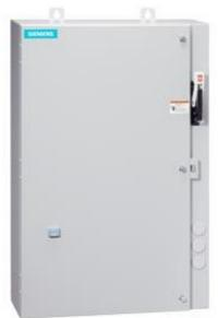
Non-reversing motor starter Size 0 Three phase full voltage Solidstate overload relay OLRelay amp range 5.5-22A 220-240/440-480VAC 60HZ coil Combination type 25Amp circuit breaker Encl NEMA type 4X 316 S-steel Water/dust tight noncorrosive Extra-wide enclosure
