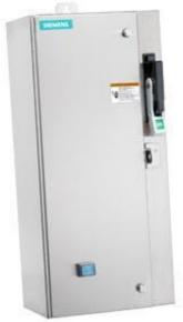
Non-reversing motor starter Size 0 Three phase full voltage Solidstate overload relay OLRelay amp range 5.5-22A 110V 50HZ / 120V 60HZ coil Combination type 25Amp circuit breaker Encl NEMA type 4X 304 S-steel Water/dust tight noncorrosive Standard width enclosure
