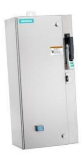
Non-reversing motor starter Size 0 Three phase full voltage Solidstate overload relay OLRelay amp range 5.5-22A 220-240/440-480VAC 60HZ coil Combination type 25Amp circuit breaker Encl NEMA type 4X 316 S-steel Water/dust tight noncorrosive Standard width enclosure
