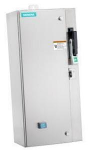
Non-reversing motor starter Size 0 Three phase full voltage Solidstate overload relay OLRelay amp range 5.5-22A 208VAC 60HZ coil Combination type 25Amp circuit breaker Encl NEMA type 4X 316 Ssteel Water/dust tight noncorrosive Standard width enclosure
